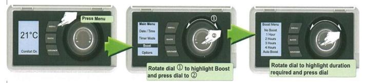
Auto Boost will automatically use the boost element to maintain the set temperature during 'Comfort On' periods.
