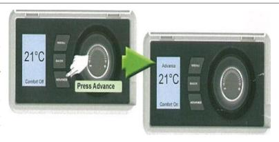
If the heater is in 'Comfort Off' mode and you want heat — press the Advance button. If the heater is in 'Comfort On' and you don't want heat, press the Advance button and it will go off until the beginning of the next 'Comfort On' period.
