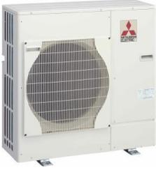
Heat energy from the outside air and mains electricity are used by the Air Source Heat Pump to heat refrigerant to a high temperature. This heat is then transferred to water which flows into your home for central heating and also for domestic hot water. The way the heat pump works is similar to a refrigerator in reverse.
